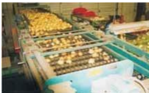
Figure.28 Sizing by rollers of increasing distance between them
