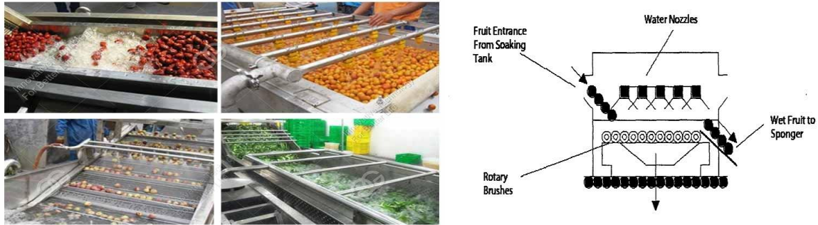
Figure. 62 Typical Produce washing machine
